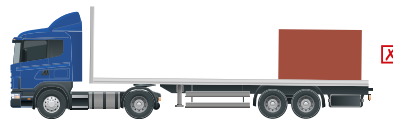
Place Cargo's center of mass in front of the center of the rear axle (group)
