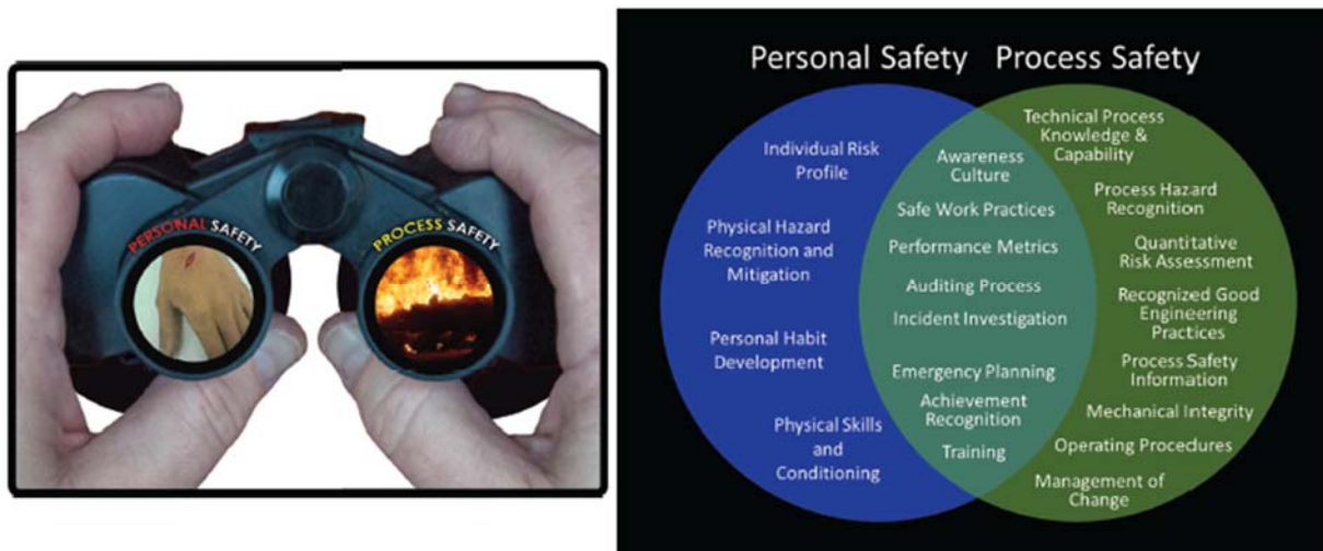
Figure I.1—Personal Safety/Process Safety Graphic
